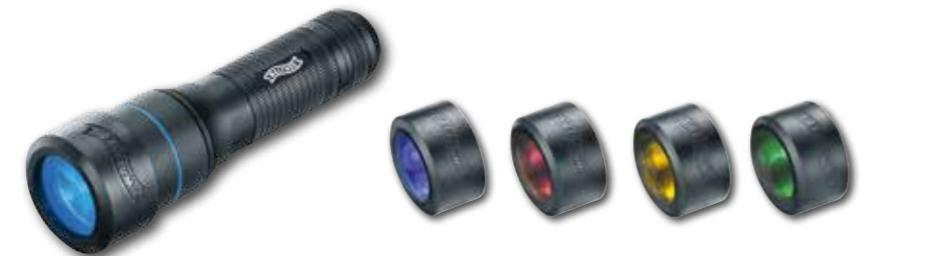
Suitable for models with a 40 mm front diameter. Four rugged glass filter discs with a special coating, 1.5 mm thick, in four matte-finished polymer collars made of rugged polypropylene. Color filters can also be used in combination with the white signal cone (Art. 3.7078). Functions: blue for better detection of body fluids (blood, sweat, etc.), red to preserve night vision, yellow for less glare in fog, green for game observation.
