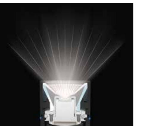
By pulling the lamp head backwards, the LED is moved far into the reflector lens. Practically all the light from the LED is projected forwards by the lens section as a wide-angle homogenous circle. This is particularly useful for the close range, permitting e.g. work without glare and non-fatiguing.
