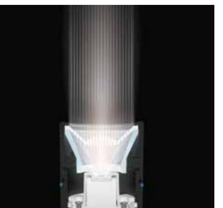
If the lamp head is pushed forwards, the LED moves to the rear of the reflector lens, thereby reducing the amount of light deflected by the lens and bundling it into a narrow beam. The remaining light is deflected by the mirror surface of the reflector, and exits the system via the transparent conical front section around the lens. Consequently, this light is not lost but is also focused, thereby increasing the luminous flux (lumens) at the focal point as well as the beam distance.
